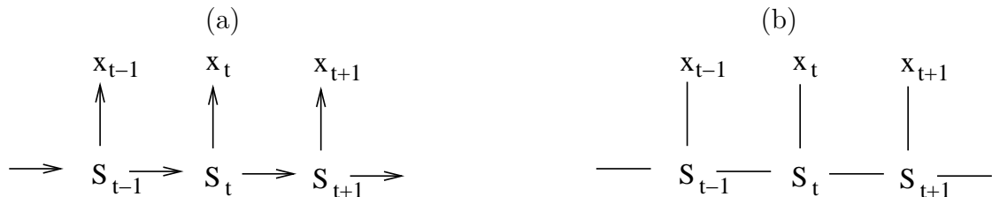
Figure 1: (a) the directed acyclic graph of the state space model and (b) its conditional independence graph.
